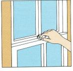
cut or removed. Window locks are an inexpensive way to keep intruders out. On double-hung windows (which slide up and down), center locks are only effective when the window is completely closed. Locks on the corners or mounted on the sides will allow you to secure windows in a partially open position.
